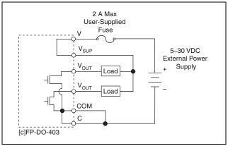
Figure 3. Wiring for Low-Current Applications
